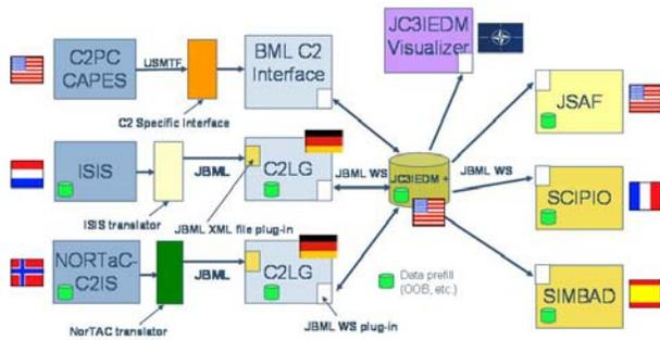
Figure 1. System Architecture
